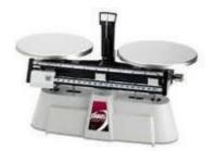
>Capacity: 2kg >Sensitivity: 1g >Two pan scale >Cast iron >Pan: 200mmØ
